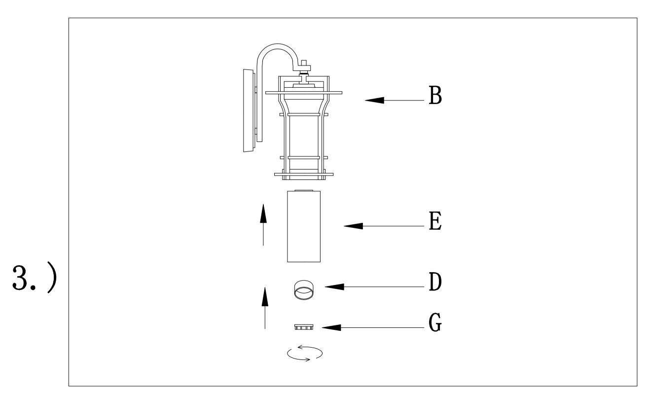
Step.3:Install the inside glass(E) to fixture(B); install the casing(D) and the screw ring(G) to fixture; Tighten the screw ring.
