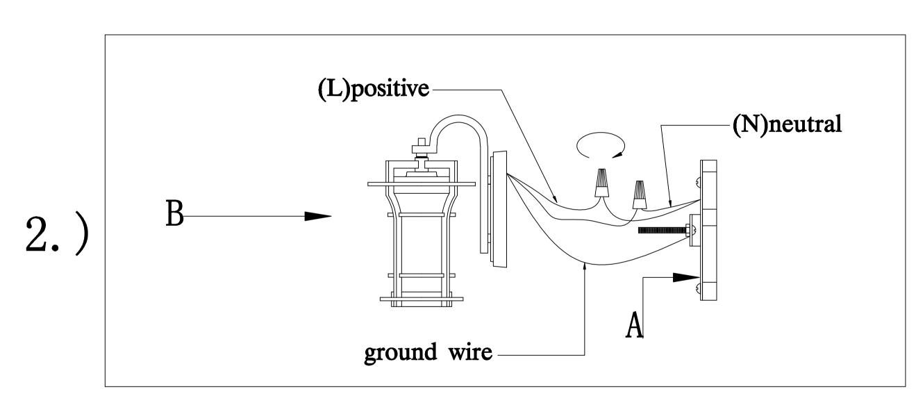
Step.2: Attach back plate to mounting bracket and tighten ball nuts so fixture meets wall. Caulk fixture where back plate meets the wall with silicone sealant.
