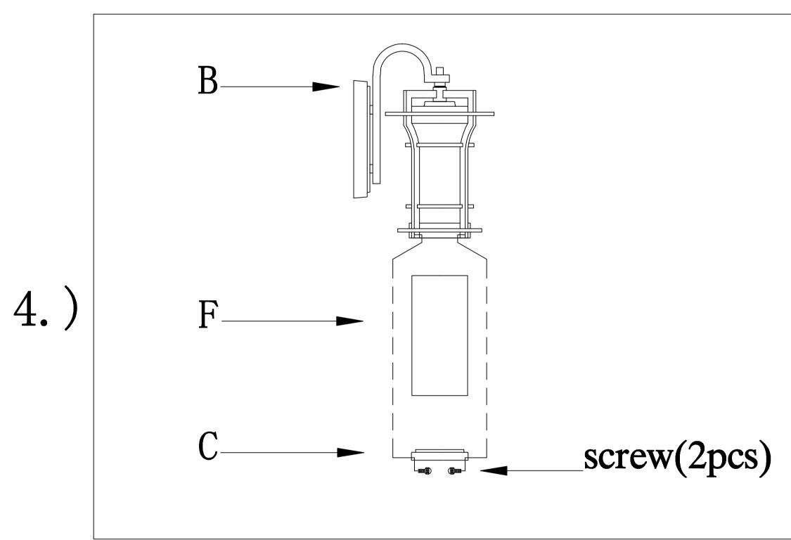
Step.4:Install the outside glass(F) to fixture; install the bottom ring(C) to fixture(B) with two screws.
