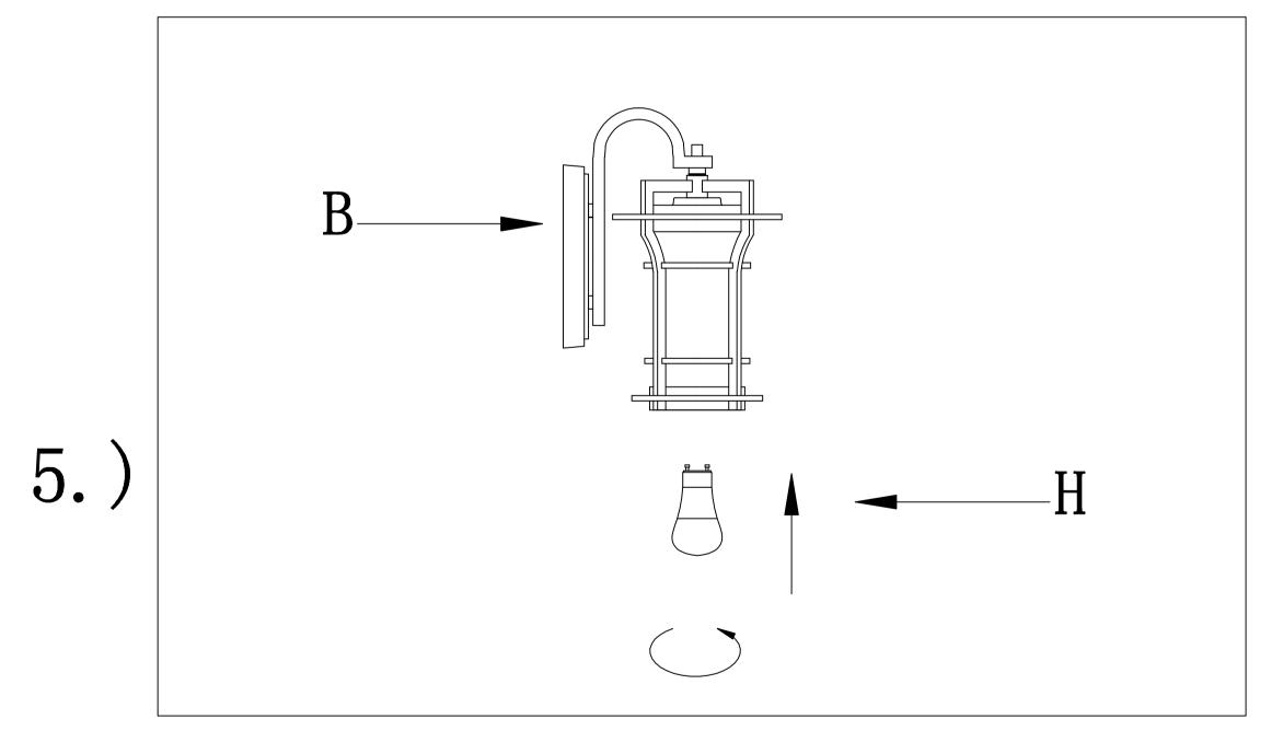
Step.5: Install GU24 LED bulb(H)
