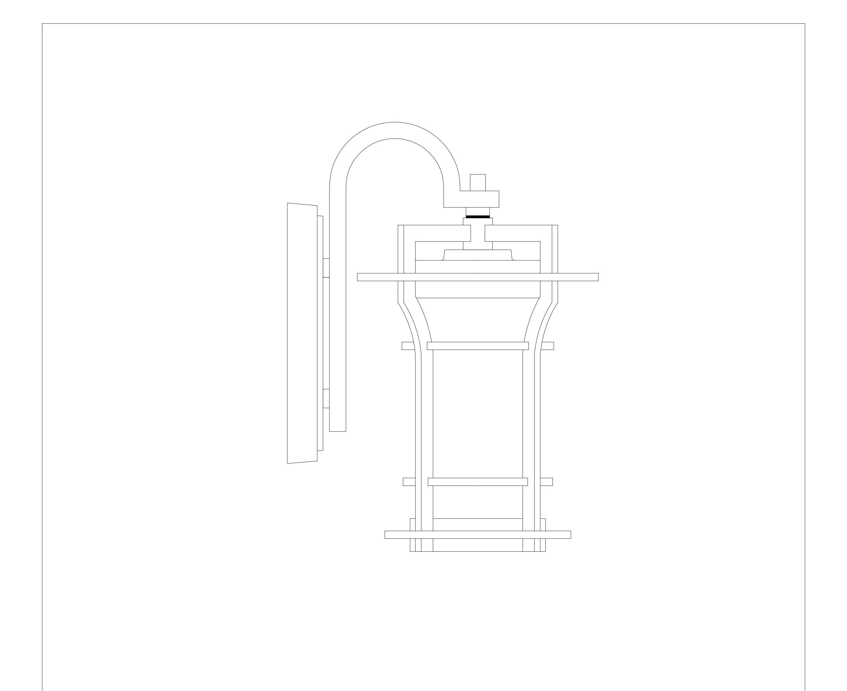
To prevent water intrusion, caulk around back-plate where fixture meets the wall using outdoor silicone sealant. Leave a small gap at the bottom to allow moisture to exit.
